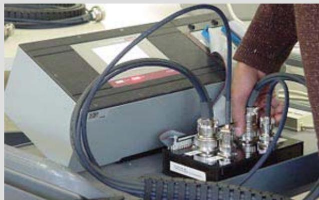
Hipot testing of newly-installed cables is standard on most projects and should be done early on before permanent power is brought into a building. It should only be performed by a qualified professional. Working with high voltage comes with risk of electrical shock, so it is important to use hipot testing equipment that meets current requirements, and to strictly follow all safety regulations and manufacturer precautions.
