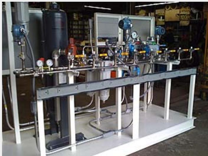
In the photos above, Omni has fabricated a breathing-air skid for one of our pharmaceutical clients. The design of this breathing-air skid is enhanced by the placement of all of the control panels to one side of the skid (left photo). The photo on the right shows full access to all valves, gauges and BA cylinders that will mount on the rear rack. In the floor of the unit are two steel-reinforced openings to accommodate a fork lift to easily rig the skid into place.
